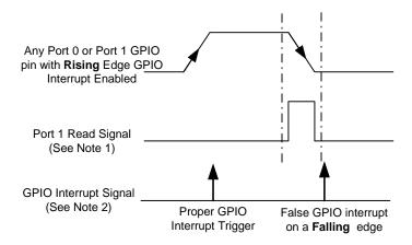
**Note 1:** Port 1 Read is an internal signal that is asserted when Port 1 is read with an "IORD 01h" instruction.
